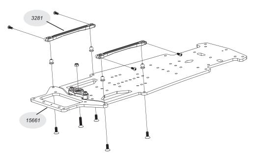
\*NOTE - Before installing, inspect the side links and you will notice that the screw holes on one side of the link are larger than the holes on the other side. Before popping the links on the balls, be sure that the larger hole faces toward the outside of the chassis.
