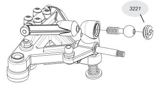
1 - Take the upper pivot ball and push it through the steering block and thread into the upper arm. Thread it in so there are no threads showing.
