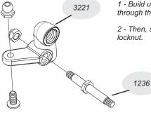
1 - Build up the left and right steering blocks as shown to the left. Start by threading the 1/4" button head screw through the steering arm of the block and into the red low profile ball.
