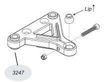
1 - Pop the brass pivot ball into the lower arm. Place the arm on a strong table and push the ball in with the back of screwdriver handle. Or preferably, you can use CRC's 4279 Ball popper pivot ball tool. Notice the "lip" of the brss pivot ball is pointing upward. The diagram to the left represents a right side lower arm. For the left side, flip the second arm over and be sure the pivot ball is installed with the lip again facing up.
