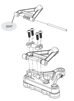
1 - Break the mold tree from the upper A-arm. You can clean up the mold gates with a hobby knife or rotary tool.
