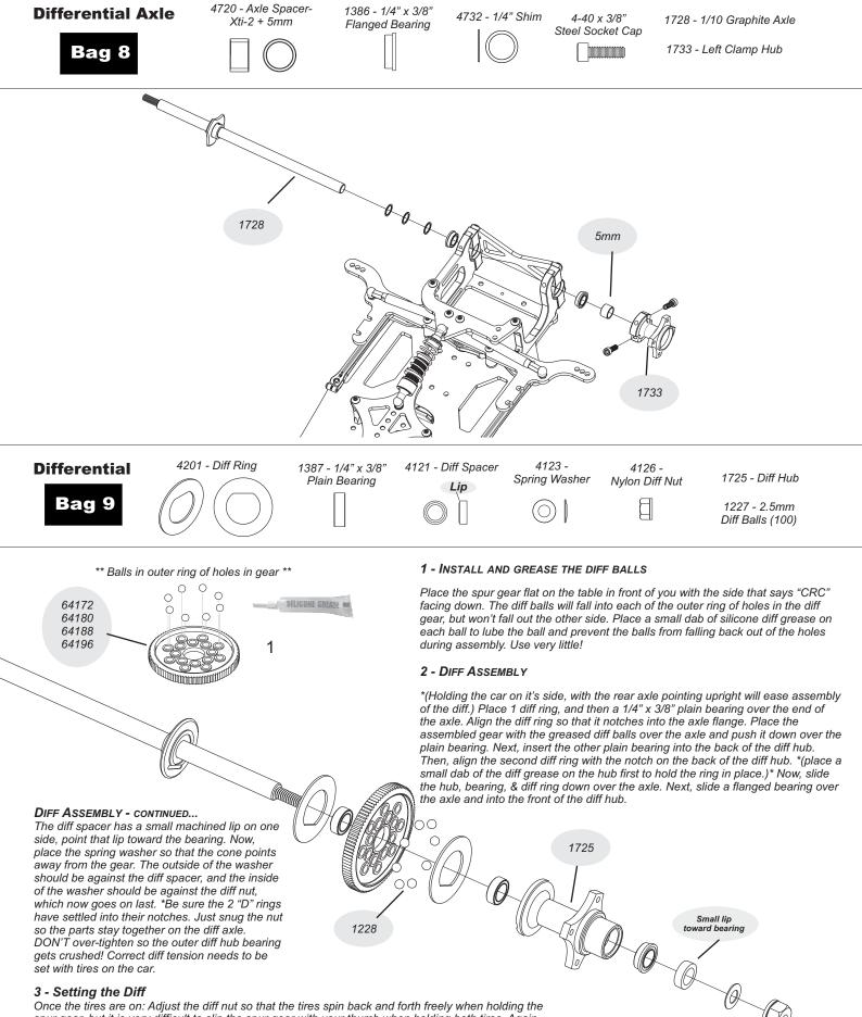
Once the tires are on: Adjust the diff nut so that the tires spin back and forth freely when holding the spur gear, but it is very difficult to slip the spur gear with your thumb when holding both tires. Again - DON'T over-tighten so the outer diff hub bearing gets crushed! Re-check diff tension after the first run.
