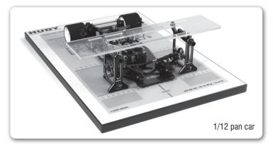
Measuring the camber and toe on a 1/10 Pan Car. (Upper adapter position is used.)
