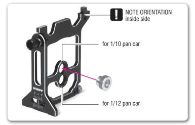
The bottom hole is for 1/12 pan cars, while the upper hole is for 1/10 pan cars. The adapter goes on the inside side of the side plate, and works as a replacement for the wheel. Therefore it is important to put it on the proper side of the side plate to keep the same width of the car.
